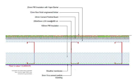
Ground floors are to be suspended steel floor cassettes, made up of Light Gauge Steel Frame Joists with 100mm PIR insulation between the steels and 25mm PIR in sulation above with a Vapour Barrier.
