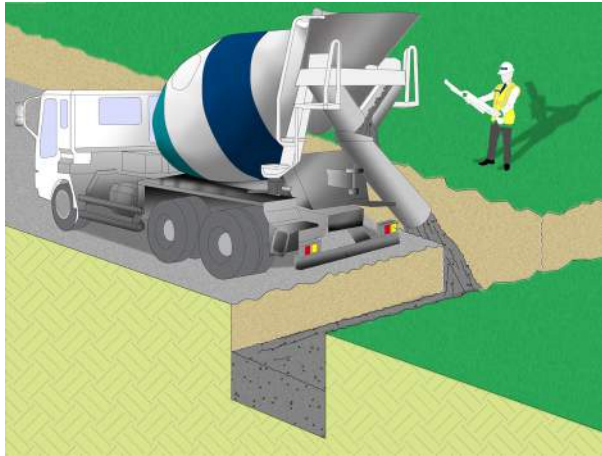
Figure 6: Ready mixed concrete
